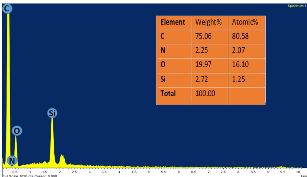
Figure 3: Energy-dispersive x-ray spectroscopy analysis of legumain-conjugated PSi.
