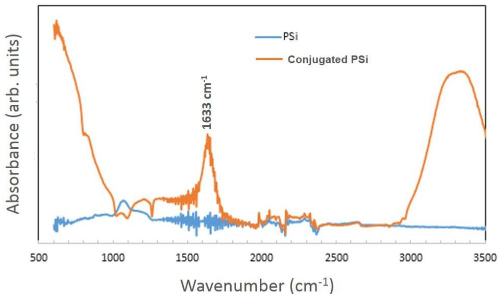
Figure 4: FTIR spectra of PSi and legumain-conjugated PSi. The PSi spectrum is nearly featureless. The sharp absorption band at  $1633\text{ cm}^{-1}$  is due to N-H vibration.
