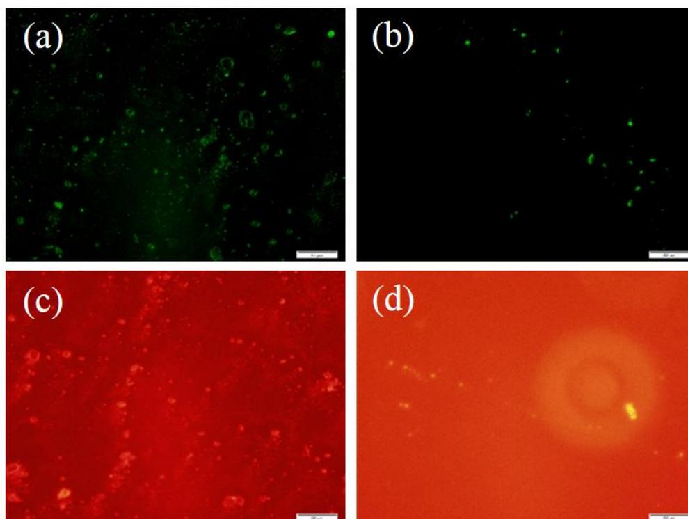
Figure 5: Fluorescence microscopy images obtained from PSi and legumain-conjugated PSi nanoparticles: (a) Pure PSi nanoparticles excited by  $\lambda = 450$  nm; (b) conjugated nanoparticles excited by  $\lambda = 450$  nm; (c) PSi excited by  $\lambda = 600$  nm; and (d) conjugated PSi excited by  $\lambda = 600$  nm. The scale bar = 50  $\mu$ m in all images.
