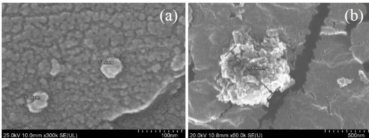
Figure 1. FE-SEM images of (a) “bare” and (b) legumain-conjugated PSi.
