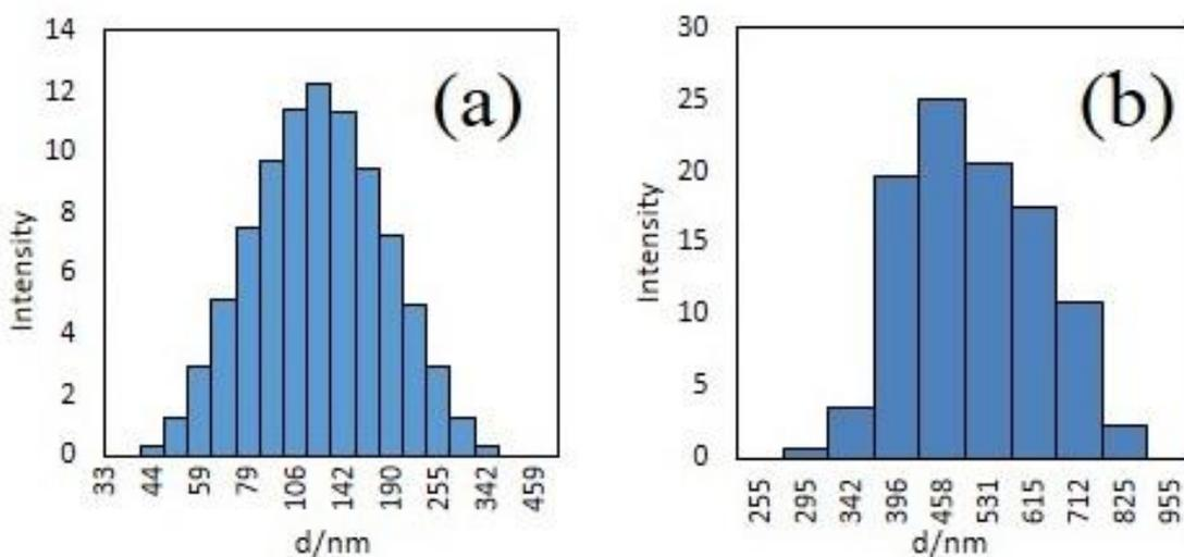
Figure 2. Particle size distribution in (a) “bare” PSi and (b) legumain-conjugated PSi obtained by dynamic light scattering.
